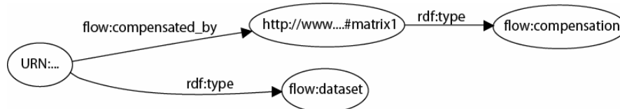
Figure 7 – A Compensation-ML file assigned to FCS data
